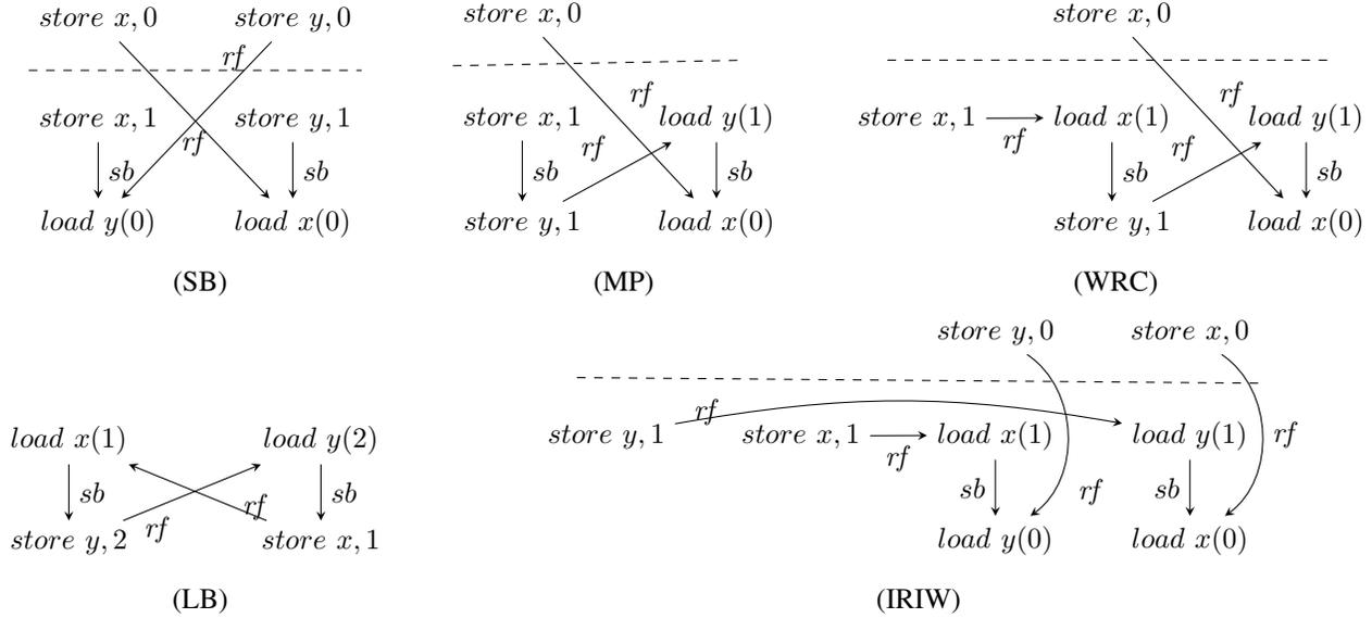
Fig. 3. Patterns of behaviors that are possible under C++ RMM but not under SC. Every column depicts the actions of one thread. We denote by *store x, l* a write of value 1 to location *x* and by *load x(l)* a read of value 1 from *x*. We assume that the initial value of *x* and *y* is 0.
