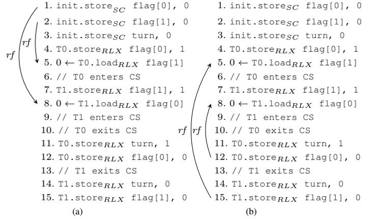
Fig. 2. An error trace containing two violation patterns: (a) store buffering (SB) and (b) load buffering pattern (LB). These patterns were detected by our tool when analyzing Dekker’s algorithm.
